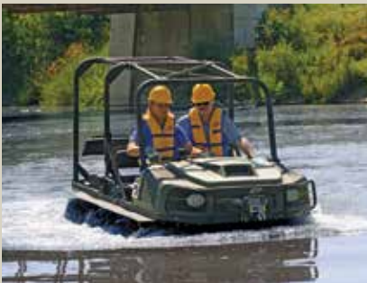
The fully amphibious ARGO can transport personnel and equipment across water and land to reach remote inaccessible locations.
