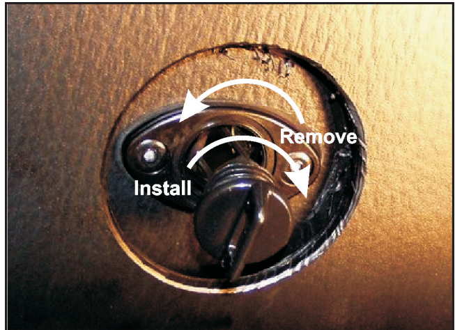
Figure 5-2. Removing and installing the drain plugs.
